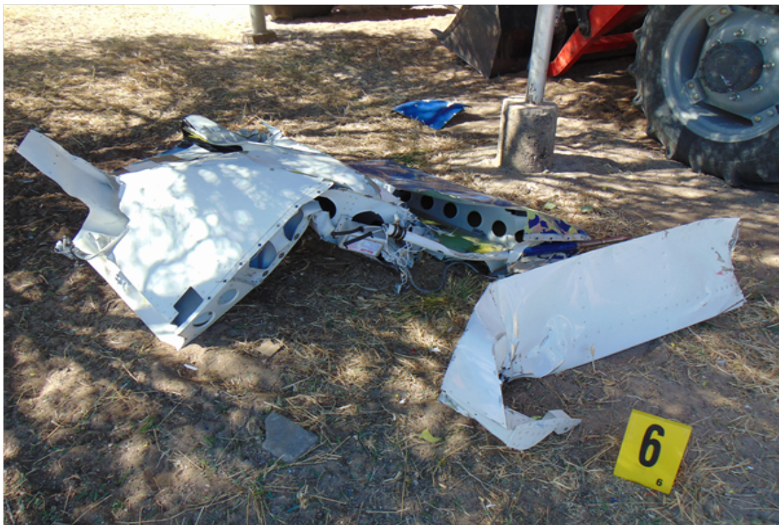
Figure 1d: Close view of the port wing tip that fell off at the spot of initial collision.
