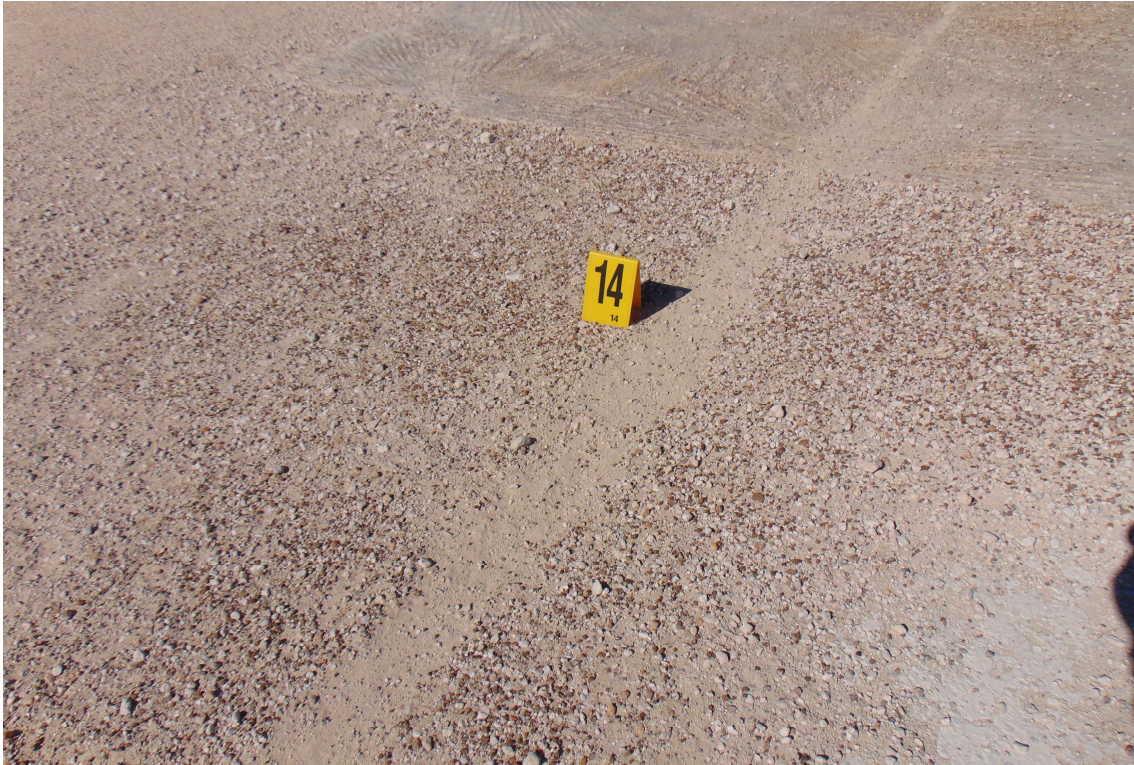
Figure 5c: Tracks of left main gear approaching the engine run-up area.
