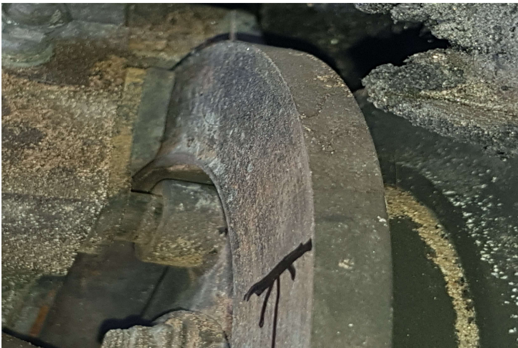
Figure 7: Picture showing main gear brake pads engaged on the disc. (Port)
