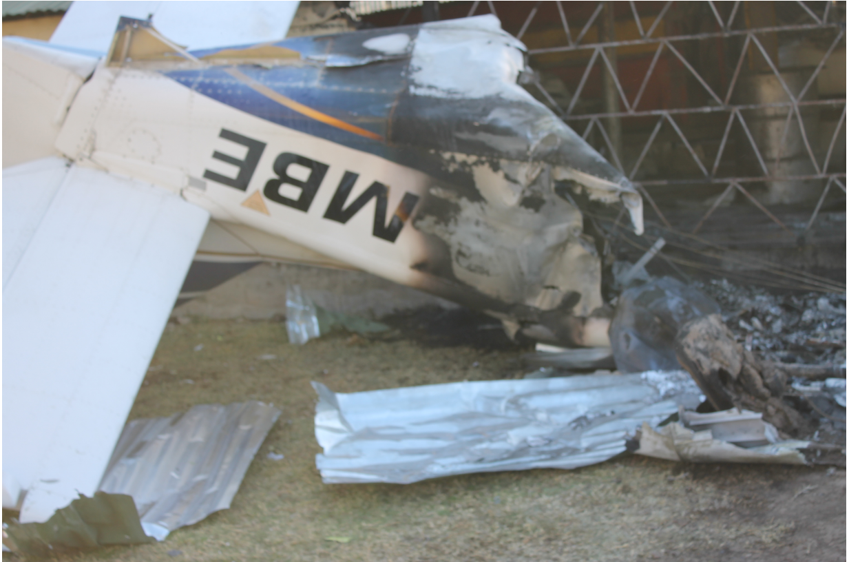
Figure 2g: View of a remaining aircraft empennage next to the farm shed.
