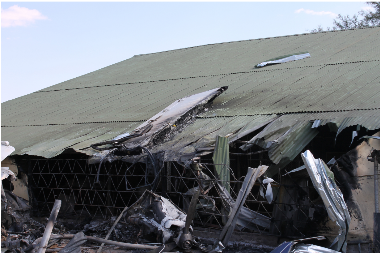
Figure 2h: The torn starboard wing resting on the farm shed roof.
