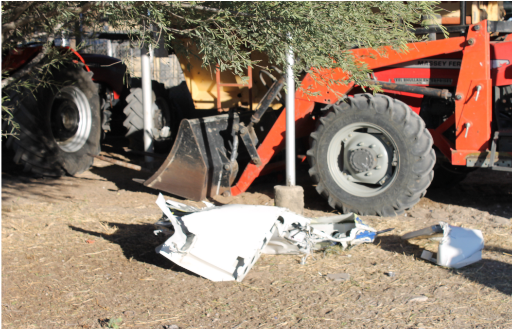
Figure 1: Images of the chopped off port wing tip that remained at the initial spot of collision.
