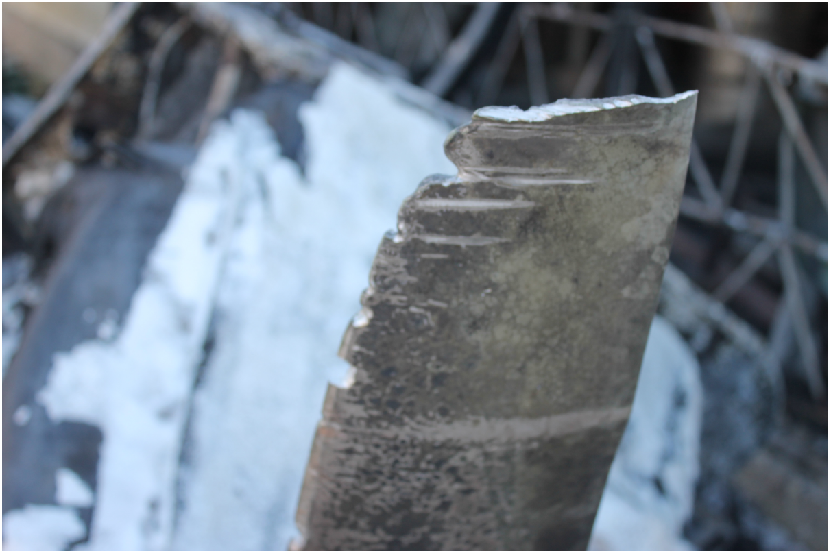
Figure 3: One of the 3 propeller blades with the tip cut off due to collision at maximum speed.
