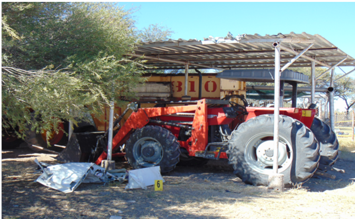
Figure 1b: View of the tree branch and the vehicle shade roof reflecting the impact from collision with port wing. (Initial points of collision).
